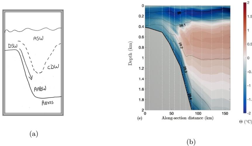
Figure 23: (a) Schematic of AABW formation and (b) measurements of conservative temperature (colors) and neutral density (black contours) across the Antarctic Frontal Structure in the Western Weddell Sea (Thompson and Heywood, 2008)
